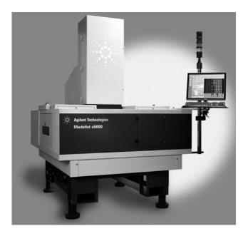
The focus of the Medalist x6000 is to reduce the manufacturers' PCBA conversion costs. In order to do this, the system provides the highest possible 3D inspection throughput, low false call rates, easy-to-use while maintaining the high level of defect coverage provided by X-ray inspection.
